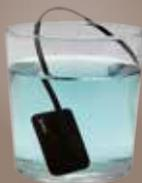
Moreover, it is completely watertight, giving you complete flexibility in your choice of disinfection method: immersion, spraying etc.
