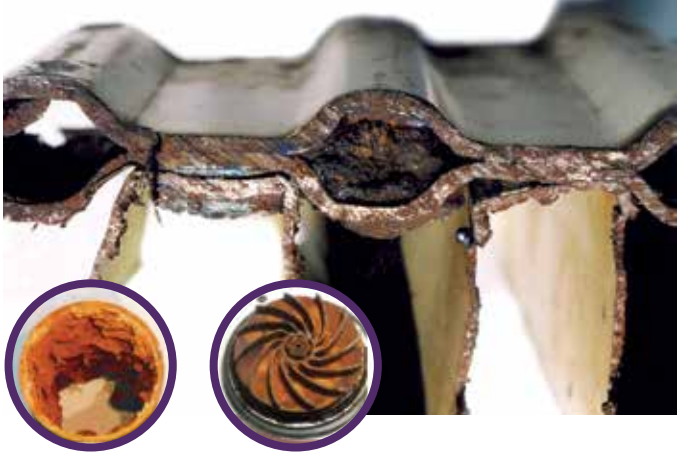
System components damaged by water contamination
