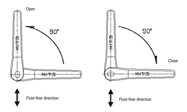
1.3 Rotation of the stem by 90 ° fully opens and fully closes the valve for Bare Stem Type. An appropriate tool or handle shall be applied to operate the valve and the flow direction shall be checked by the top orientation of stem.
