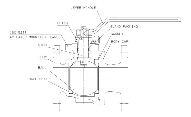
This illustration introduces a typical construction.
