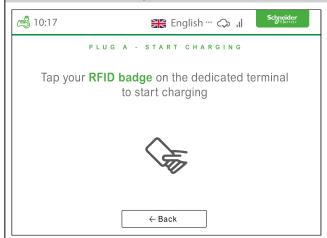
A • After inserting the vehicle connector in the Electric Vehicle port the user interface will prompt the user to tap the RFID card.
