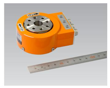
The SLP-NA-T is a strain gauge based load cell for simultaneous measurement of forces in three mutually perpendicular axes. Since the load cell is constructed small and light, it is well suited to use in model testing.
