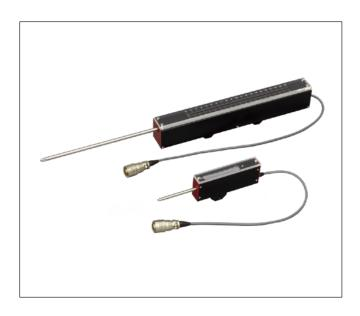
This is a strain gauge type displacement transducer for general purpose. This transducer has a small cantilever inside, and displacement is mechanically converted into deflection of the cantilever. Strain, which is proportional to the deflection, is generated on the cantilever and is measured by strain gauges. Stable measurement is possible even for a small displacement. The scale and pointer on the main body enables easy positioning of the transducer.
