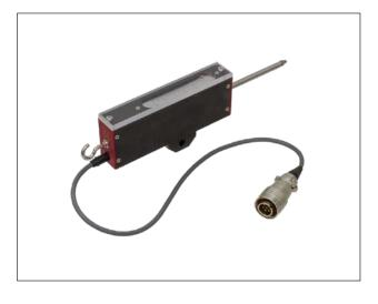
This is a strain gauge type displacement transducer for general purpose. This transducer has a small cantilever inside, and displacement is mechanically converted into deflection of the cantilever. Strain, which is proportional to the deflection, is generated on the cantilever and is measured by strain gauges. Stable measurement is possible even for a small displacement.
