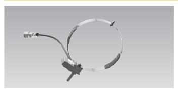
The OU displacement transducer is a combination of a round plate spring and strain gauges. It is mounted with its contact tip pressed against a structure. When displacement occurs in the structure, the plate spring is deformed and the amount of output proportional to the amount of displacement can be output.
