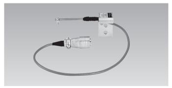
The CE displacement transducer has the structure of strain gage mounted on a cantilever. The high responsiveness to displacement and the simple structure allows this transducer to make accurate and stable measurement and to be installed in a confined space.
