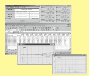
The Visual LOG Light is a control software of monitor-alarm with use of our static strainmeters. With different computer interface and such instruments, the software consists of 4 models, -1. TDS-700L for GP-IB/RS-232C, -2. TDS-701L for MODEM(Telephone modem), -3. TDS-702L for Modem-DM( Data Logger data memory) and -4. TDS-703L for TRG(Wireless Telemetry modem).
