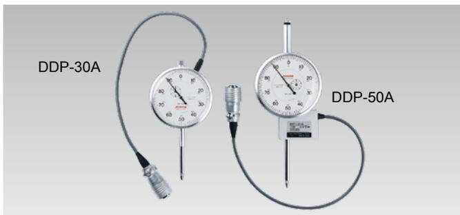
The DDP-A displacement transducer is a dial gauge with a strain sensing element and a bridge circuit integrated. The amount of displacement can be checked by viewing the pointer while the output from the sensing element can be used to control a recorder or a machine.
