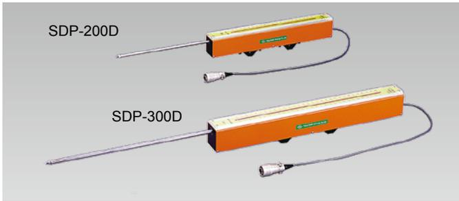
The SDP-D displacement transducer is an axial type transducer with a measuring range of 200 mm or 300 mm. The strain gauge type design makes this transducer free of the noise generated by sliding electrical contact points. Taking advantage of the stroke of the axial part, it can measure a large amount of displacement and make stable measurement over a long period of time. As it is provided with graduations, alignment work can be done easily.
