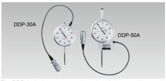
The DDP-A displacement transducer is a dial gauge with a strain sensing element and a bridge circuit integrated. The amount of displacement can be checked by viewing the pointer while the output from the sensing element can be used to control a recorder or a machine.
