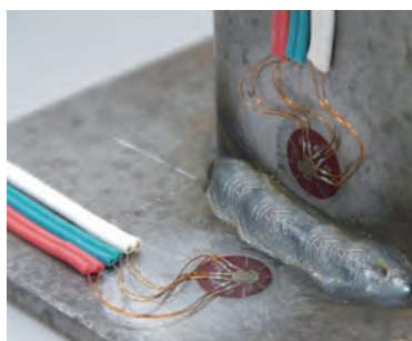
Weld bead (rosette strain gauge)
