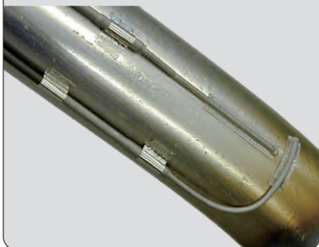
R: Bend of gauge backing or pipe
