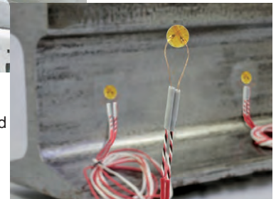
Railway axle load measurement
