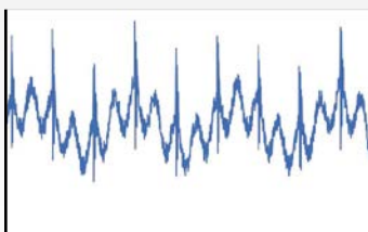
Waveform affected by noise
