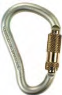
RGK3 EN362 Material - steel Gate opening – 22mm Size – 125mm x 90mm Closure type – twist lock MBS – 40kN Weight – 276g
