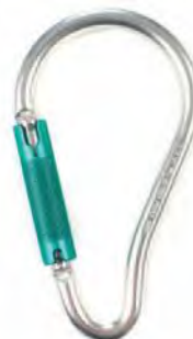
RGK6 EN362 Material - aluminium Gate opening – 53mm Size – 235mm x 130mm Closure type – twist lock MBS – 23kN Weight – 348g
