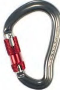
RGK4 EN362 Material - aluminium Gate opening – 25mm Size – 125mm x 90mm Closure type – twist lock MBS – 28kN Weight – 85g
