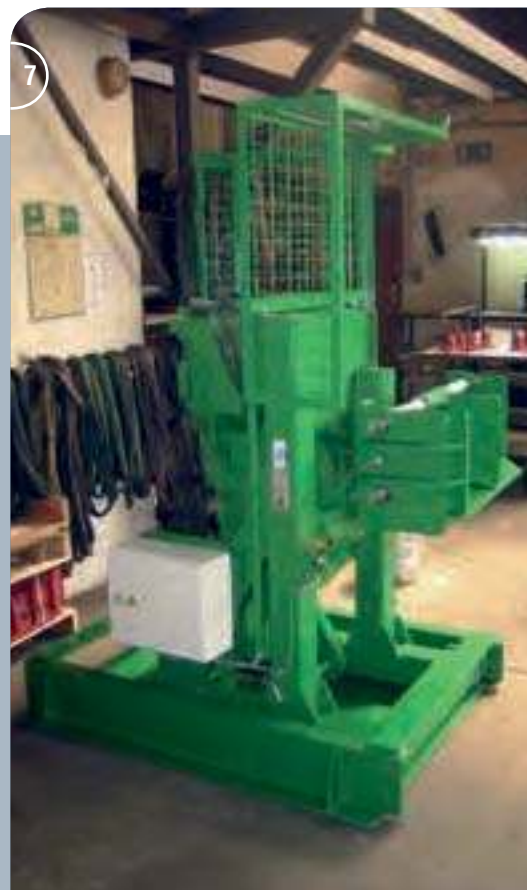
7 Elektromotorische Trägerwendevorrichtung für Walzprofile. Electromotive beam turning equipment for rolled steel sections.
