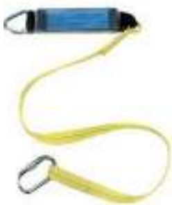
RGL1 EN354 and EN355 44kN polyester webbing Length 1.3m and 1.8m Shock absorber pack Maximum arrest force <6kN
