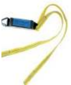
RGL3 EN354 and EN355 Twin leg lanyard 44kN polyester webbing Length 1.3m and 1.8m Shock absorber pack Maximum arrest force <6kN
