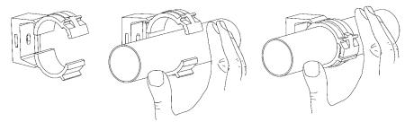
Simply mount CLIC, push pipe in by hand, grips and locks by applying slight pressure. To open: unlock the CLIC latch with screwdriver.
