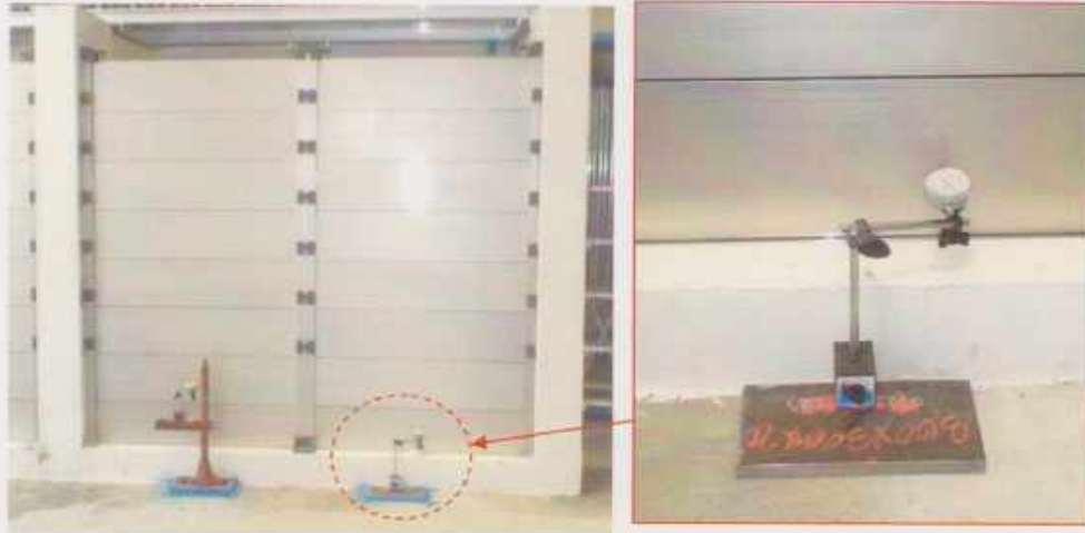
Fig. 1.3 Installation of Dial indicator for pressure resistance test at point No.1
