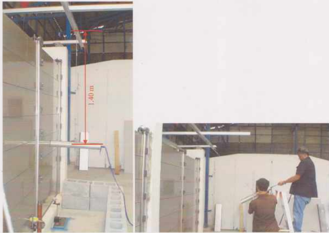
Fig 2.2 Equipment preparation for hit resistance test using the vertical distance of 1.40 m from the hanging point to the middle of the steel block (at the center of 4 th sheet from the bottom).
