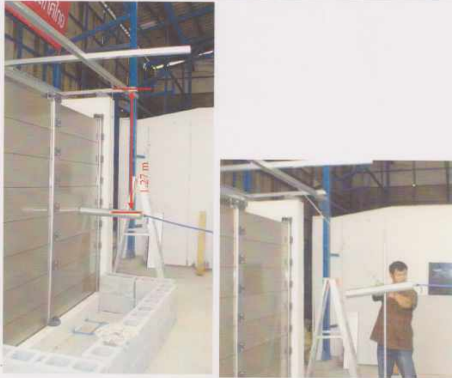
Fig 2.1 Equipment preparation for hit resistance test using the vertical distance of 1.27 m from the hanging point to the middle of the steel block. (at the junction of 4 th sheet and 5 th sheet from the bottom).
