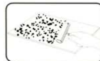
Sweep the dirt on the Tacsil surface out using Ethanol immersed roller
