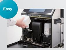
Easy and quick replacement of ink and makeup cartridges without staining your hands. A new error prevention feature (alarm) is provided using IC tags for ink and makeup replacement. Simplified checking makes the replacement more effective. \*Some geographic areas are excluded. Convenient LITACHI IJP
