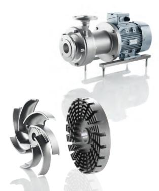
This magnetically coupled pump is designed for applications with special safety requirements. The FPM / FSM is specifically suited for transferring toxic, dangerous or water-hazardous goods. The open impeller is connected to the driving unit via a magnetic coupling that is contact-free. The pump's product space is hermetically sealed from the environment by a separating can.
