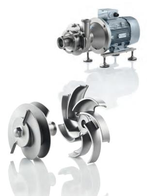
This newly designed pump offers superior performance with gaseous liquids and in CIP return applications. It combines Fristam's proven impeller with a rotor screw. This clever design results in a low-noise hybrid that pumps liquids with significant gas content at high efficiency. The FPC is also suitable for emptying tanks.
