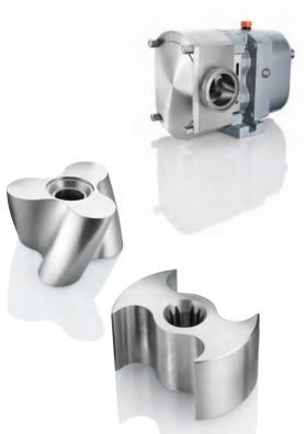
The FL is universally suitable for many standard applications. It is hygienic, gentle, low-maintenance, durable and economical. The Fristam FL3 features unique helical three-winged rotors and is specifically designed for revolution speeds of up to 1,000 min<sup>-1</sup> as well as for CIP return processes. This saves you an additional pump in a bypass line. All models are compact, very easy to clean as well as fully capable of CIP and SIP.
