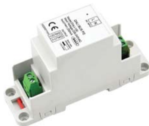
DALI BUS PS (IP20) (DALI BUS Power Supply) 11.2 x 3.5 x 6.7cm (105g) • The 1 CH DALI Power Supply 250mA • Plug and play : Simple structure and easy to operate, plug and play
