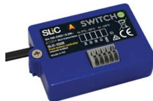
SLiC550E (IP20) (Push button controller) 6.1 x 4.2 x 2.1 cm (25g) Wire Length : 20M (max) • Easily configured by the Casambi App to provide on/off, Smooth Dimming, lighting Scene, Colour or Animation control.
