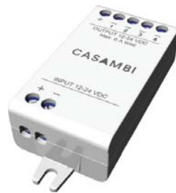
CBU-PWM4 (IP20) (4-Channel PWM Dimmer) 7.26 x 3 x 1.8 cm (23g) • สำหรับ Linear / Strip Light Dim / CCT / RGB / RGBW • Max. output power 144 W (24 VDC) 72 W (12 VDC)
