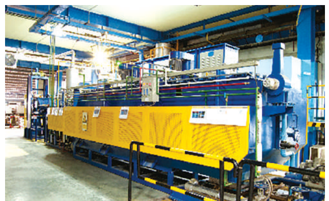
In house Heat Treatment process by Austempering for spring property
