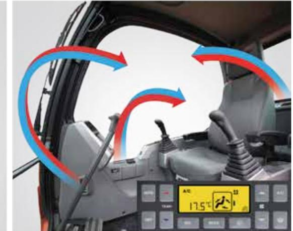
The high performance air conditioning provides an air flow which is adjusted and electronically controlled for the prevailing conditions. Five operating modes ensure even the most demanding operator will be satisfied.
