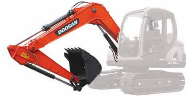
The boom lower plate is designed as an integral type to reduce weld joints and stress concentration. The thicknesses of the side and upper plates of the arm have been increased for further reinforcement.
