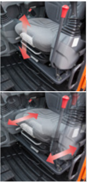
Adjustable seat, head rest and arm rests For more operator comfort.
