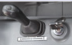
Dozer float function and travel mode switch
