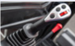
Proportional joystick with auxiliary thumb control
