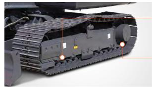
The track roller attachment point was shifted from lower to middle portion to improve undercarriage stability and structural rigidity of the chassis.
