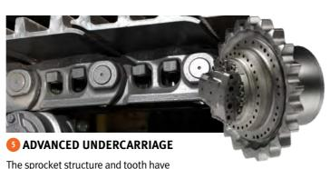
The sprocket structure and tooth have been strengthened to prevent debris and increase durability.
