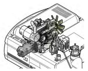
Engine & pump matching, the new technology of Doosan, fully resolves problems; low respones time of the system, unnecessary fuel consumption. Matching response time between pump and engine efficiently reduces unnecessary fuel consumption as well as exhaust fumes.
