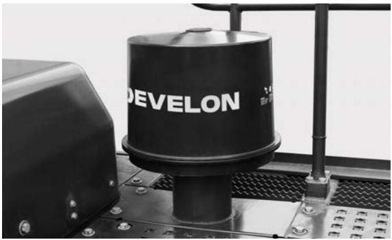
PRE-CLEANER Rotor type dry pre-cleaner attached as a standard option.
