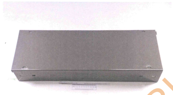
Sample after 24-hours salt spray test
