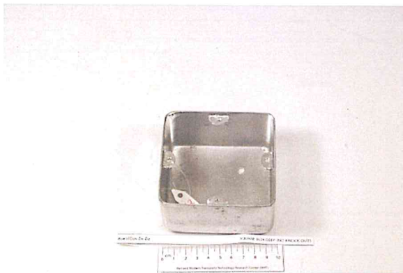
Sample before salt spray test
