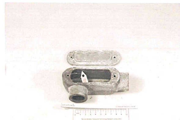
Sample after 24-hours salt spray test
