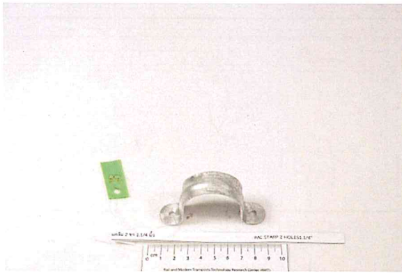
Sample before salt spray test
