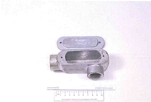
Sample before salt spray test
