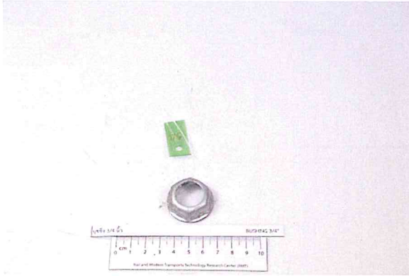
Sample before salt spray test
