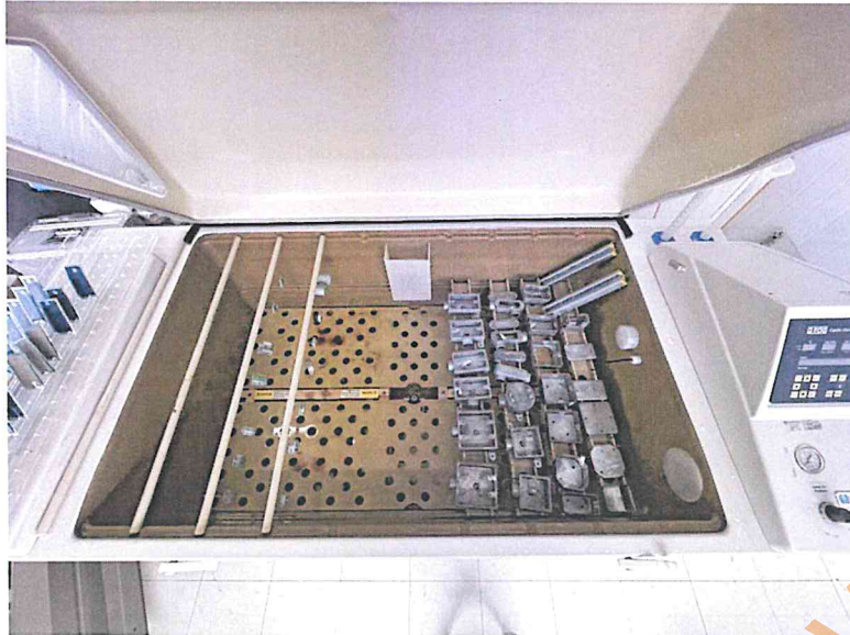
Fig. 1: Samples of electrical conduit fitting used to test corrosion resistance by the salt spray technique.
