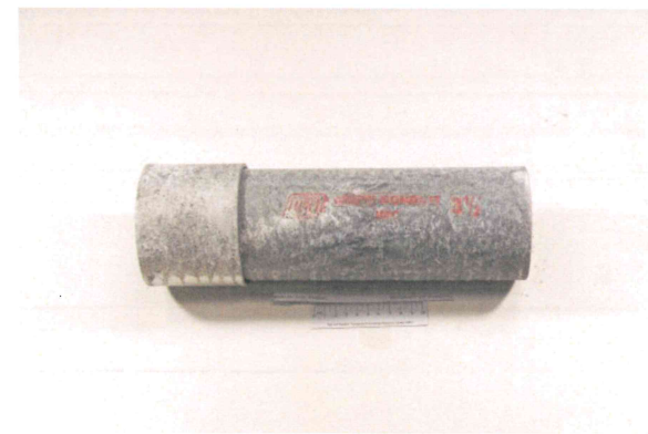
Sample after 24-hours salt spray test
