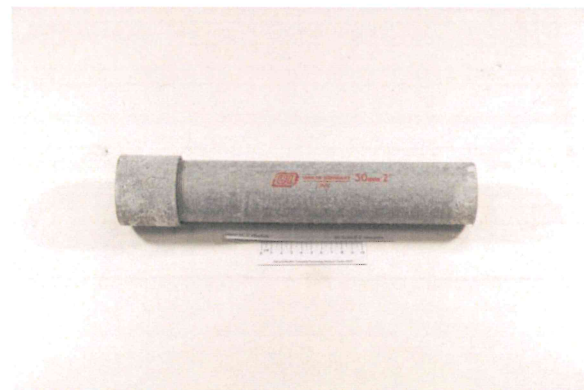
Sample after 24-hours salt spray test
