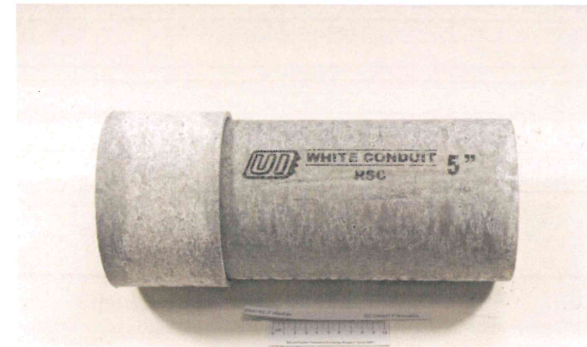
Sample after 24-hours salt spray test
