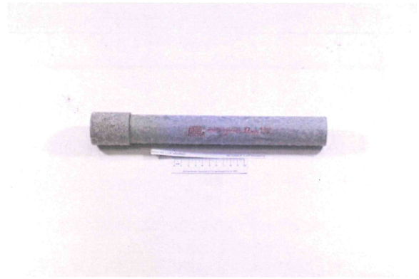
Sample after 24-hours salt spray test
