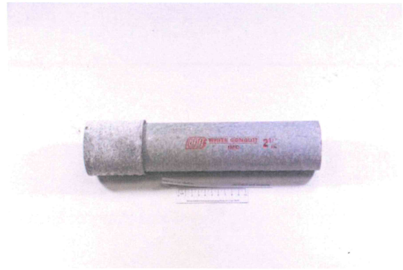
Sample after 24-hours salt spray test
