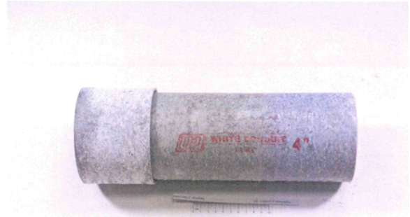
Sample after 24-hours salt spray test
