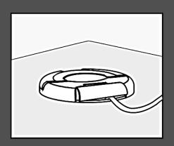
2. Press the master switch on. A green light confirms that power is available. You can use all the power sockets.
