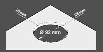
Cut-out a 92 mm diameter hole in the work surface and allow a minimum of 25mm clearance surrounding the cut hole.
