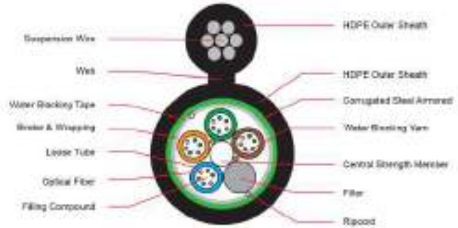
Fig.8, Multi-Tube, Armored UFCX8XXMA
