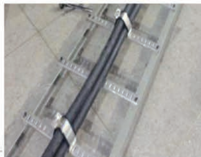
IEC61914:2009/9.5 Short-circuit test ( 180kA )
