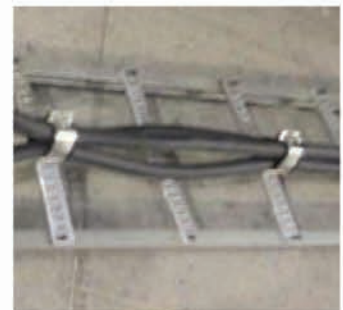
IEC61914:2009/9.5 Short-circuit test ( 180kA )
