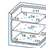
ASTM standard, 12 points testing
