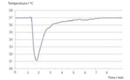
The temperature rise curve to 37°C after opening the door for 30 sec at 22°C ambient temperature.
