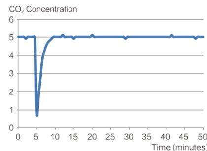
CO<sub>2</sub> concentration recovery curve (door open for 30s)
