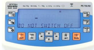
Display has a new text information line allowing to show additional messages and data
