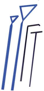
L-shape The traditional spreaders are used for spreading bacteriological cultures evenly. The shape allows the user to rotate and apply easily throughout an entire round plate or dish. They are made of ABS and have a slight upward curve at the edge to prevent dragging or scraping.
