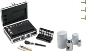
Accuris calibration weights are ideal for routine calibration of your Accuris (or any brand) lab balance. Single weights as well as complete weight sets are available in various tolerance classes: OIML class E2, F1, and M1.
