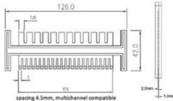
Large teeth: 5.65x1mm, well volume 22.6µl for 0.5mm thick gel Small teeth: 3x1mm, well volume 12µl for 0.5cm thick gel 3mm wide teeth taper from 2mm to 1mm at tip
