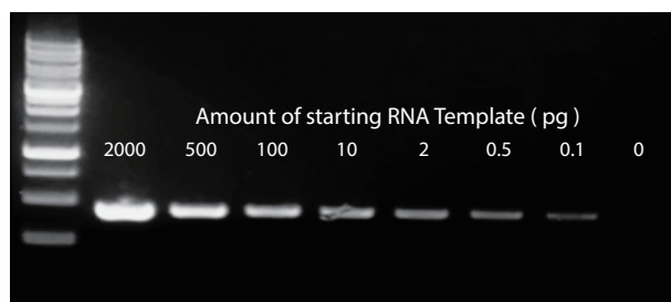
Figure 4: Sensitivity of OneScript® Reverse Transcriptase PCR amplification using human cDNA synthesized with OneScript® with varying amounts of starting RNA (2000 pg - 0 pg), followed by electrophoresis on a 1% agarose gel.
