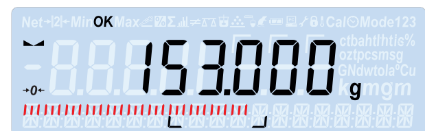
Mass value contained within thresholds
