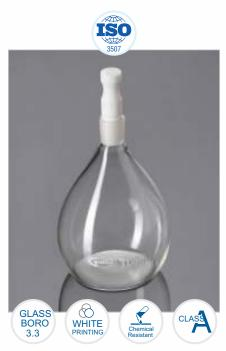
BOD Bottles for incubating diluted samples of clean water, waster water, effluent water and polluted water during the 5 day biochemical oxygen demand (BOD) test. These BOD bottles feature a flared mouth to form a water seal to prevent the ingress of air during incubation. The interchangeable stoppers have a tapered bottom that also prevents air entrapment.
