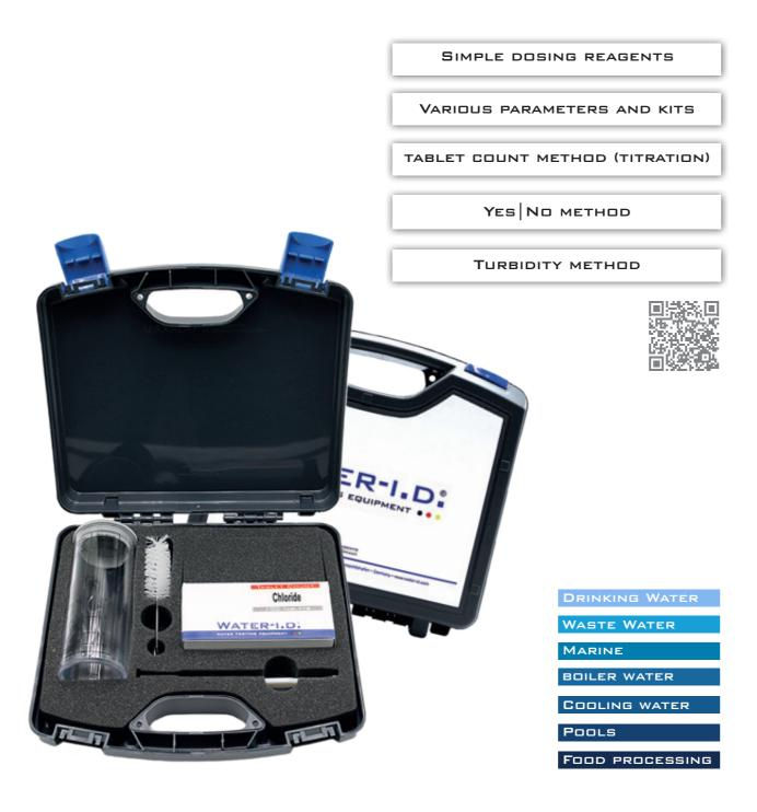
Some Water-i.d.® Mini Kits are based on the tablet counting method, in which tablets are added to the water until the colour changes in a defined way. The amount of added tablets is entered into a formula to determine the measured value. The innovative Water-i.d.® tablet pushthrough blisters simplify the procedure.
