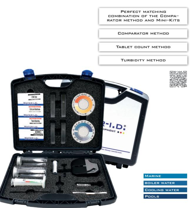
Balanced Water Kits are a perfect matching combination of the Comparator method and Mini-Kits, such as the tablet count method and the turbidity method, covering many important water parameters in one kit.
