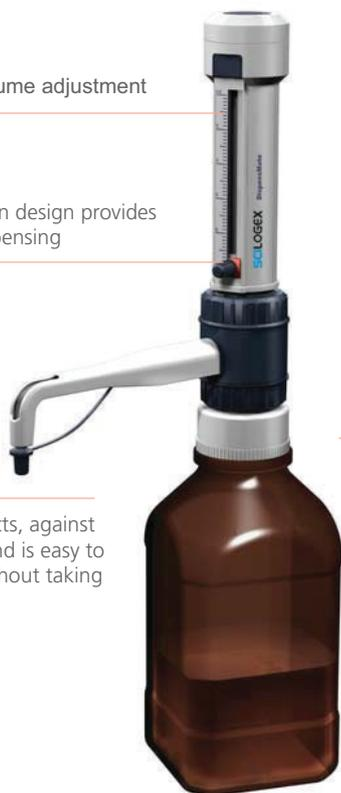
6 Adapters allow fitting to standard reagent bottles
