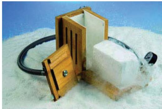
The '**SCIOGEX**' Portable Dry-Ice maker is the fastest way of providing a block of Dry-Ice to your lab. It is compact and lightweight, requires no electric power and is safe and simple to use. Most importantly, it is always there in the lab to give you immediate access to Dry-Ice WHEN YOU NEED IT. The economy of having your Dry-Ice 'on tap' can provide considerable financial savings over a relatively short period as the cost of having Dry-Ice delivered to your lab can be prohibitive.
