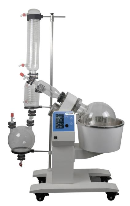
The SCI20L-Pro is ideal for continuous distillation of many volatile solvents under reduced pressure. It offers an excellent distilling solution in a wide range of applications.
