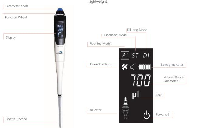
iPette is an innovative electronic pipette developed by SCILOGEX. It combines the features of manual pipette and ergonomic and lightweight.
