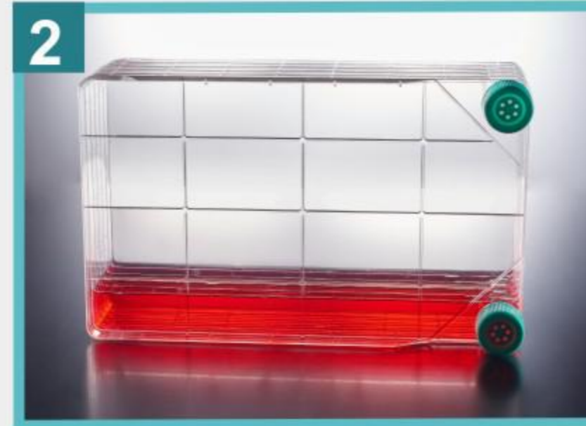
2 Equilibrate by placing the Cell Factory system on the side with the small port
