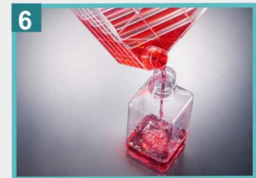
6 Loosen the cap and empty directly into the reservoir
