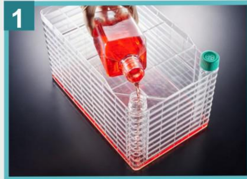
1 Pour the media directly into the Cell Factory system
