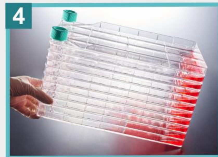
4 Carefully tilt the Cell Factory system to a horizontal incubation position with the filling inlet up
