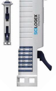
SCILOGEX repeater pipette tips are particularly suitable for dispensing of fluids with high viscosity, high vapor pressure etc. Tips are made from high-quality materials (Cylinder: PP, Piston: PE-HD) without soft lubricants or other additives.
