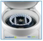
Unique **COMBI-Rotor**<sup>™</sup> Accepts tubes and strips
