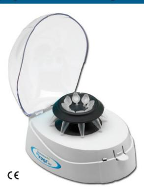
The myFuge<sup>™</sup> Mini Microcentrifuge is a personal centrifuge that virtually fits in the palm of your hand. Ideal for quick spin downs of microtubes and PCR tubes, the myFuge is extremely easy to use. Simply close the lid and the rotor instantly reaches 6,000 rpm. Open the lid, and the improved braking system quickly and smoothly decelerates the rotor to a complete stop in just one second.
