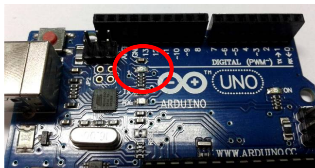
Figure 8. The position of LED L on Arduino Board circuit
