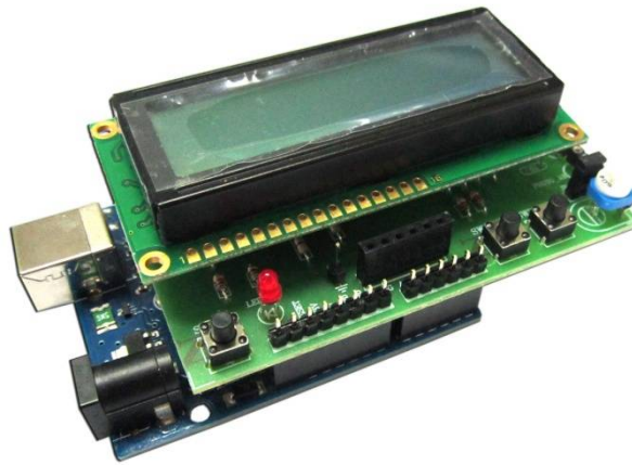
Figure 9. Connecting FK1416 board with Arduino UNO R3 board
